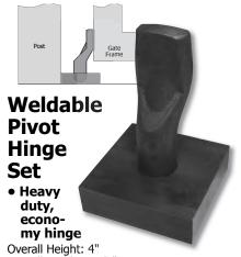
Overall Width: 2-1/2" sq. Pin: 7/8" dia. x 3-7/8" length Base: 2-3/4" x 2-3/4 x 3/4" thick Base plate is machined from solid steel. Hinge pin is weldable cast iron.
